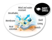
Softshell with TPU membrane consists of three layers. Due to the microporous TPU membrane as middle layer the material is water-proof, wind-proof and breathable at the same time.
