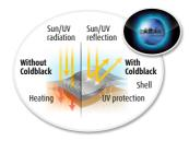
Textiles with a coldblack®-finish afford optimum protection against heating up through sun rays. They stay cooler and protect reliably against UV rays (min UPF 30). The effect of this is that the person wearing these garments does not sweat so easily, feels better and is even more efficient. coldblack® is a registered trademark of Schoeller Technologies AG,
